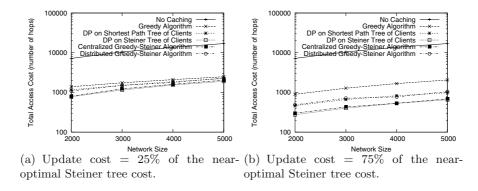
Fig. 2. Access cost with varying number of nodes in the network for different update cost constraints. Transmission radius  $(T_r) = 2$ . Number of clients = 50% of the number of nodes, and hence increases with the network size.
