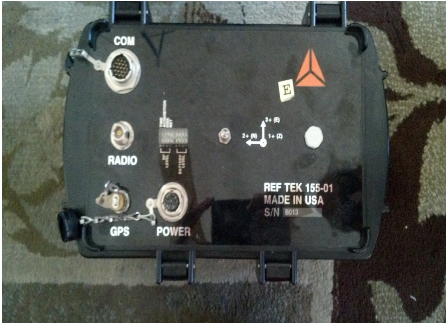
An external view of Shake Box, showing GPS, POWER, Radio Com Port etc.
