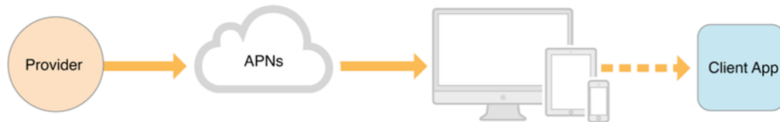
Figure 2.2.1: Structure and Flow of Apple's Push Notification Service [4]
