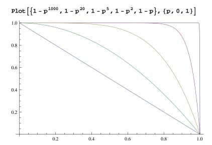
An increase of probability of not fail of a system relative to probability of not fail for a single disk as a function of probability of fail of a single disk.
