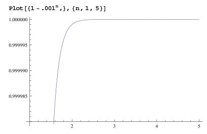
Probability of not fail of the system as a function of n, given the probability of fail of 1 disk = .5
